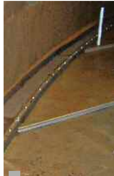
CTS' IFR wiper seal after more than 10 years in service
